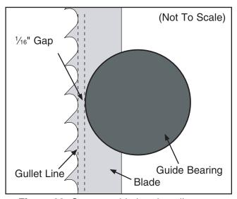
**Figure 32.** Correct guide bearing alignment against the blade.
